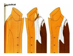
Fig.7-17: Shoulder pad attaching
