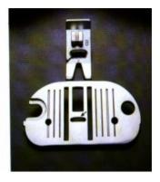
Fig.4-5: Straight-stitch and zigzag plates and feet
