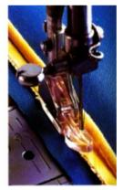
Fig.4-6 Zipper foot, seam guide and blind stitch hem foot
