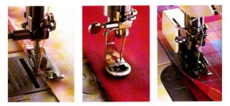
Fig.4-7: Even feed, button and over edge feet
